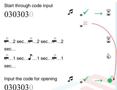
If a delay time has been programmed, this must be started first by inputting a valid opening code. It can then be opened by inputting any desired valid user code during the time window for opening.
